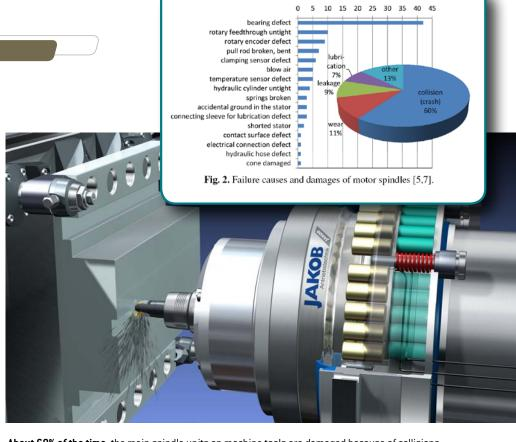
About 60% of the time, the main spindle units on machine tools are damaged because of collisions.
