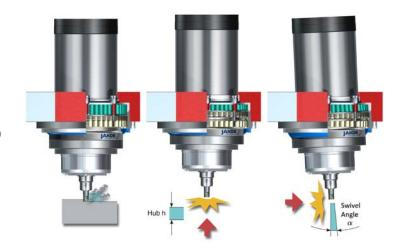
**The collision protection system** from Jakob Antriebstechnik, Kleinwallstadt, Germany, and marketed in North America by GAM LLC is based on a double-flange design.
