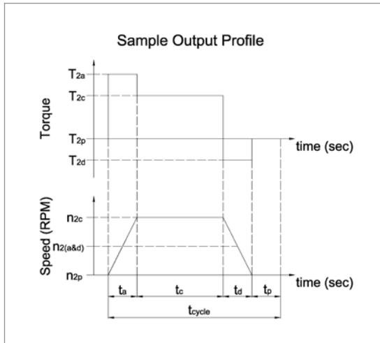
$$ED = \frac{t_a + t_c + t_d}{t_{\text{cycle}}}$$
